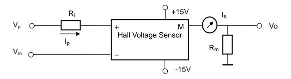
A magnetic field is generated by current  $I_p$  when a voltage  $(V_p\text{-}V_m)$  is applied on the input terminals of the sensor through the primary resistor  $R_i$ . This magnetic field is compensated with the reverse magnetic field caused by the current  $I_s$  in the secondary coil. The field compensation effect can be detected with a Hall Effect element. One obtains the following equation when the magnetic flux is zero:
