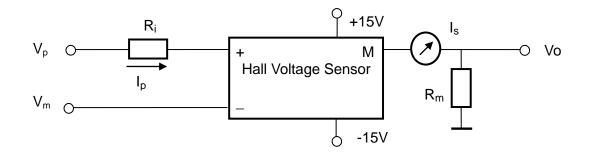
A magnetic field is generated by current  $I_p$  when a voltage  $(V_p-V_m)$  is applied on the input terminals of the sensor through the primary resistor  $R_i$ . This magnetic field is compensated with the reverse magnetic field caused by the current  $I_s$  in the secondary coil. The field compensation effect can be detected with a Hall Effect element. One obtains the following equation when the magnetic flux is zero:
